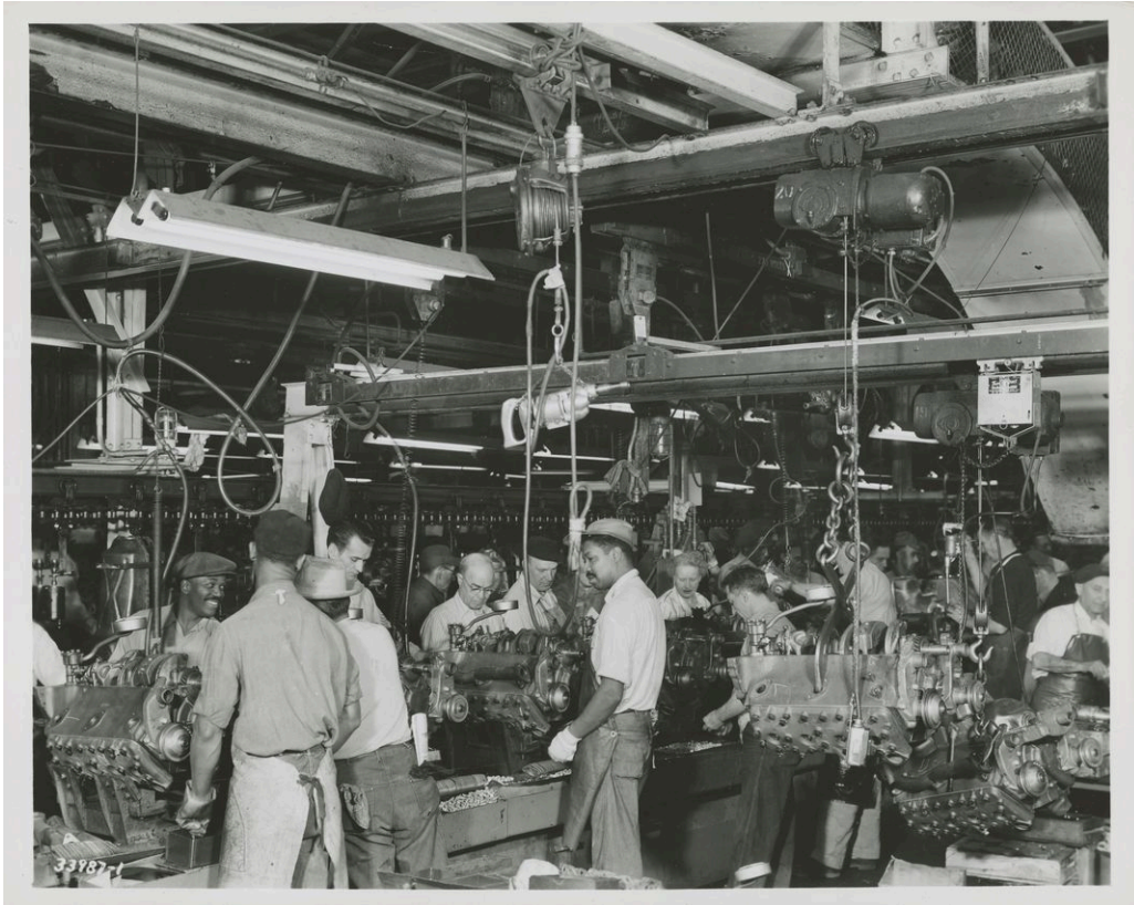
Engine assembly at the River Rouge plant in January 1948 The Henry Ford
